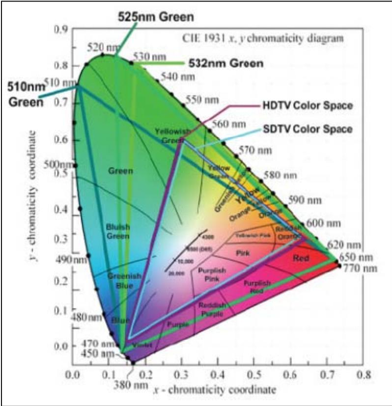
Figure 3 – Chromaticity advantages of 4-laser Systems with two green lasers
