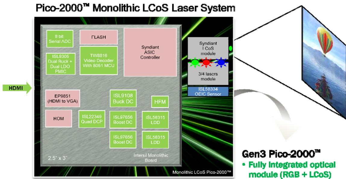
Figure 4 – High-Performance Laser-based Pico Projector Reference Design
