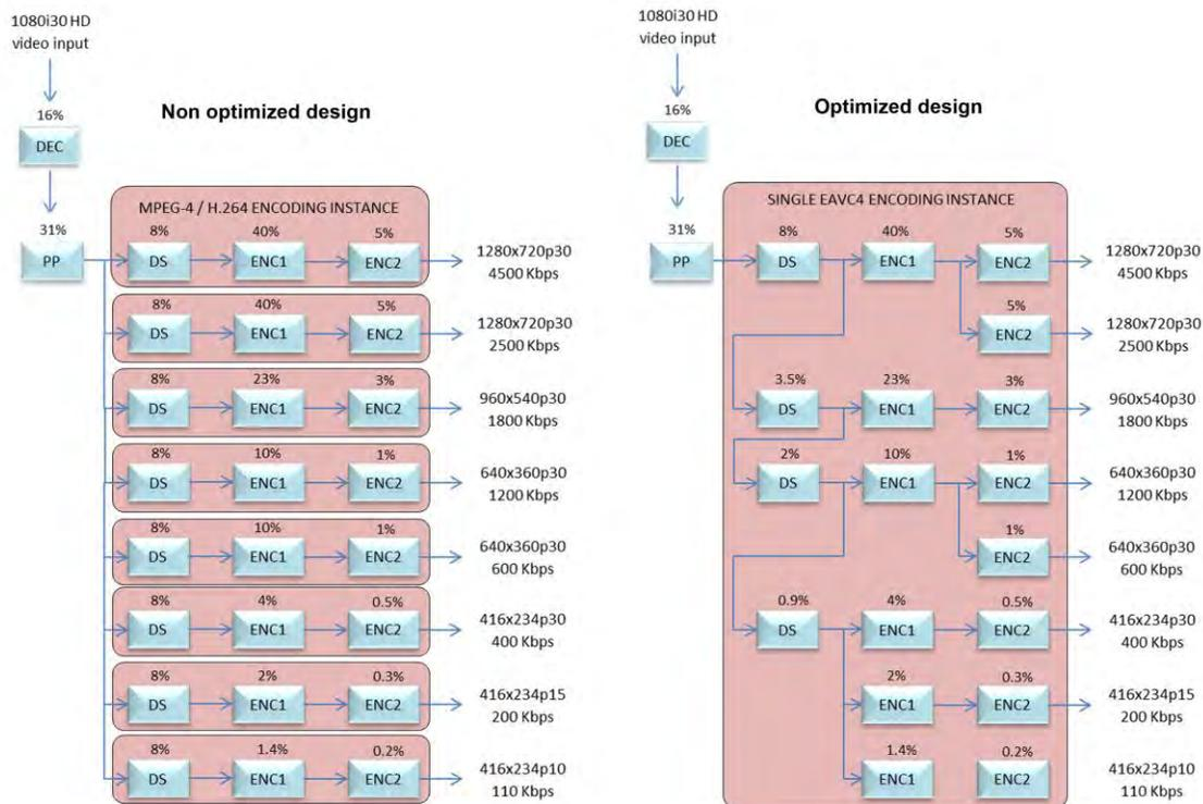
Figure 7 – Video Encoding Pipeline Optimization with “Multi-screen by Design”
